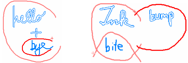
Fig. 12. Left: Circle of exclusion; the user lassos hello+bye then recircles bye to exclude it from the selection. Right: Adding to selection with a bump and removing with a bite.
